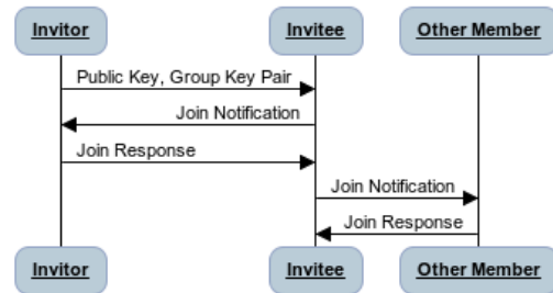
Figure 2: Any group member can invite new participants by sharing the group key pair and a partial list of group members with another Musubi user.
