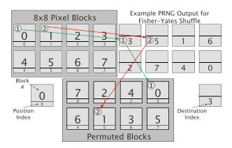
Figure 3: Example of 8×8 block permutation.
