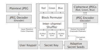
Figure 1: The ESP encryption architecture for JPEGs.
